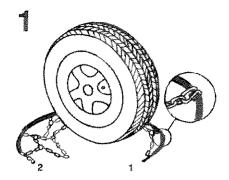
Lay the chain on the ground making sure that it is not entangled and that the open ends of the double hooks are facing the ground. Pass one side of the cable and chain behind the wheel.
