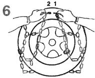
Unhook the ends of the cable (1 and 2)
