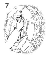
Attach the rubber tensioner to equal segments of the side chain, as shown.
