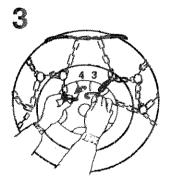
Pull the side chain to the center of the tire. Attach the side chain over the flat hook. (3 and 4)
