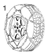
Stop the car so that the flat hook (3) on the side chain is at the top center of the wheel.
