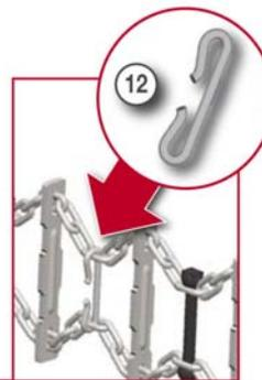
(UK) If necessary remove this special hook to elongate the chain
