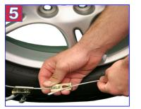
5) Grab the outside cable with both hands and pull it towards you to create as much slack as possible; then take the NUB end of the lower outside cable (near the ground) and thread it through the lower keyhole fastener.
