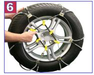
6) Attach rubber adjuster equally to each of the six sections of the outside cable to tighten the additional slack. To make this process easier, attach the first hook of the adjuster at the 1 o'clock position, the next hook directly opposite the first, at the 7 o'clock position and so forth. Hooks on the rubber adjuster should be facing away from tire.
