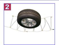
2) Lav cable chain on ground with smooth side of the cross member hooks (stamped "Tire Side") facing up. Move the chain in a sweeping motion under the vehicle so the chain continues around the backside of the tire.
