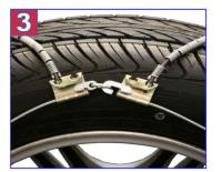
3) Reach around the back of the tire with both arms and grab both ends of the non-split side cable that is furthest away from you. Pull both ends to the top of the tire so the fasteners can be seen and handled easily. Fasten the rear side cable by connecting the quick hook to the chain link.
