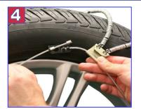
4) Next, center the cable chain on the tire so that each side cable extends equally down the sidewalls of the tire. At the top front of the tire, take the NUB end of the outside side cable and thread it through the key hole fastener.
