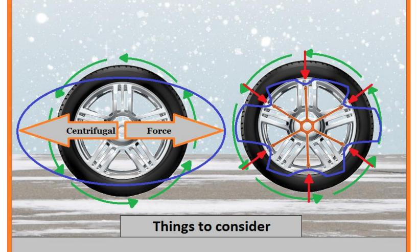
During the normal use of a tire chain, the steel can stretch. This is due to the movement associated with the chain rotating and pulling causing the chain to become slightly larger on the tire over time. Using a spider bungee will pull the extra slack out of the chain evenly. This minimizes the force when the chain contacts the ground surface reducing the effects of wear.
