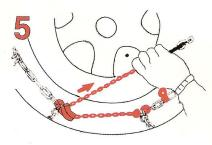
Pass the red tensioning chain through the groove of the red locking device (6) Pull the tensioning chain in the opposite direction tightly securing the chain on the tire.
