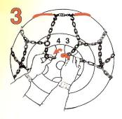
Pull the side chain to the center of the tire. Attach the side chain over the flat red hook. (3 and 4)
