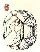
Pass the rubber cord through the red shortening ring and hoot it firmly to the side chain.
