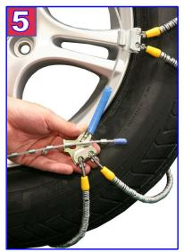
5) Grab the outside cable with both hands and pull it towards you to create as much slack as possible; then take the "Nubbed" end of the lower outside cable (near the ground) and thread it through the gold key hole fastener. Make sure that both fasteners (top and bottom) are adjusted within one "Nub" of each other.
