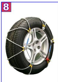
8) Chain tighteners and/or adjusters should not be used on the High Volt. Box 8 shows a High Volt chain that has been correctly installed.
