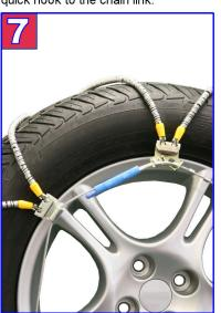
7) To secure the "Nubbed" ends of the outside cable, move the blue spiral plastic over them using a turning motion.
