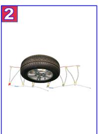
2) Lay cable chain on ground with smooth side of the cross member hooks (stamped "Tire Side") facing up. Move the chain in a sweeping motion under the vehicle so the chain continues around the backside of the tire.
