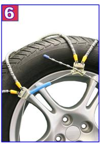
6) Move the vehicle forward or backwards 5 - 10 feet. Re-tighten both fasteners as equally as possible to remove any excess slack.
