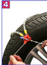
4) Next, center the cable chain on the tire so that each side cable extends equally down the side walls of the tire. At the top front of the tire, take the "Nubbed" end of the outside cable and thread it through the red key hole fastener.
