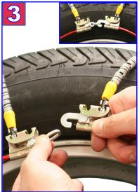
3) Reach around the back of the tire with both arms and grab both ends of the non-split side cable that is furthest away from you. Pull both ends to the top of the tire so the fasteners can be seen and handled more easily. Fasten the rear side cable by connecting the quick hook to the chain link.
