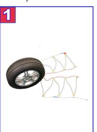
1) Park vehicle on level ground and away from traffic. Set emergency brake. Chains are to be installed on drive axle wheels (example: rear wheel drive, place chains on rear tires. Front wheel drive, place chains on front tires.)
